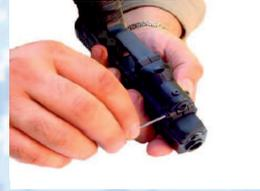
Insert and tight the mount to housing fixing screws **REMEMBER NOT TO OVERTIGHT**
