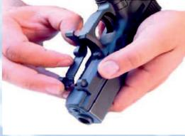
Install the two mount sides making sure to match the internal rail to the frame.
